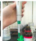
Figure 8: Pipette pen used to extract and measure the crosslinkers in microcentrifuges.
