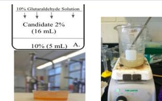
Figure 14a-B: Shown here is the interface schematic (A) and the final crosslinked interface product (B).
