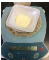
Figure 4: Weighing of the bovine gelatin powder for the 2% gel base.
