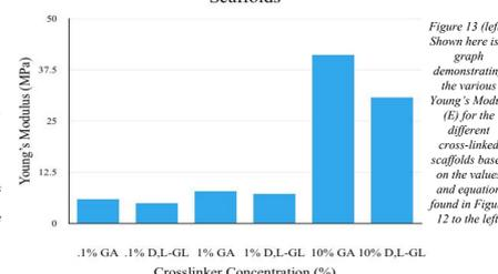
Figure 13 (left): Shown here is a graph demonstrating the various Young's Moduli (E) for the different cross-linked scaffolds based on the values and equation found in Figure 12 to the left.
