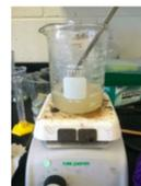
Figure 15: Formulating of the 10% bovine gelatin base with use of a hot place to help dissolve gelatin powder faster.
