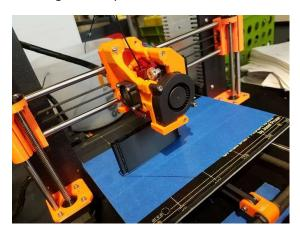
The other item we requested was for an upgrade for a new extruder head (flexion) for the 3D printer. Of the 14 students who worked in my lab, 7 benefitted from the upgrade on the 3D printer. A picture of the new extruder is also included above.
